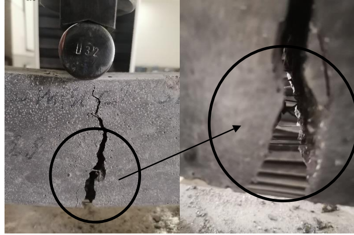
Fig. 17. Performance of steel fibers in FRC under flexural loading.
