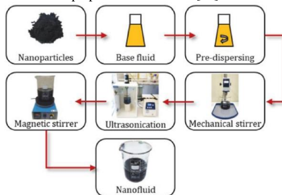
Figure 4. Schematic diagram of two-step process to prepare the nanofluids methods [59]
