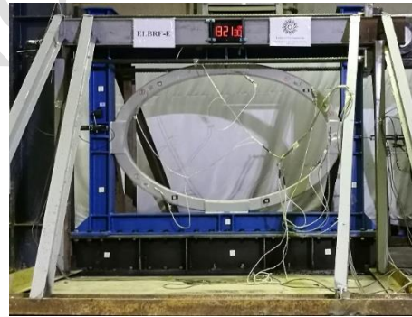
Fig. 14. Tests on elliptic-braced frames [41-42]
